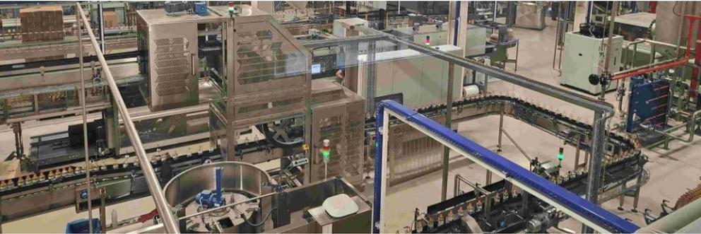
The facility operates two fully automated bottling lines designed to ensure high precision, consistency, and operational efficiency. These lines are fitted with dry conveyor systems to reduce moisture-related risks and safeguard product integrity, as well as enclosed conveyors that further enhance food safety by minimizing contamination risks and ensuring compliance with stringent industry and regulatory standards.
